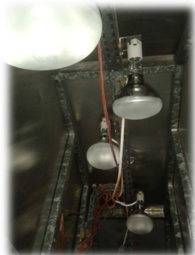
Figure 14 : Lampes Ultra Vitalux
