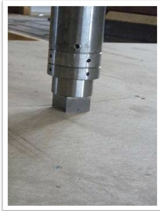
Figure 3 : Application de la charge au joint
